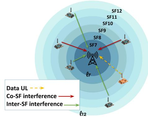
Fig. 1. LoRa system, with end-devices transmitting simultaneously
